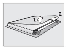
■ **Gently** lift the inner pane up and pull out of the cover strip.
